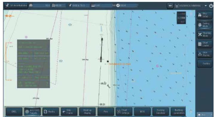
**Activate the prediction** to monitor the calculated future position based on Rate of Turn and Heading of the vessel.
