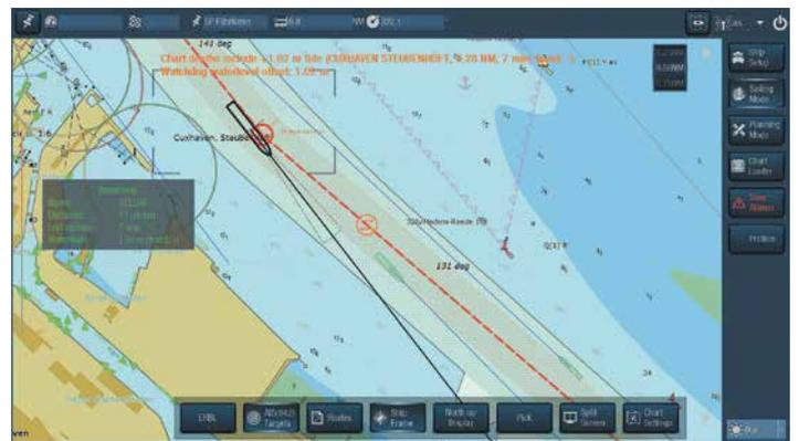
**Online Water Level Correction** for direct depth correction in the chart and Watchdog settings.
